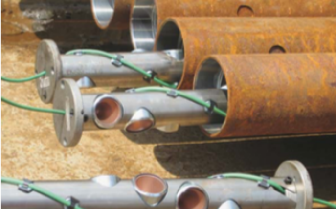
Figure 6: Cylindrical Perforating gun in pipes (Thomas & Alan, 1982)
